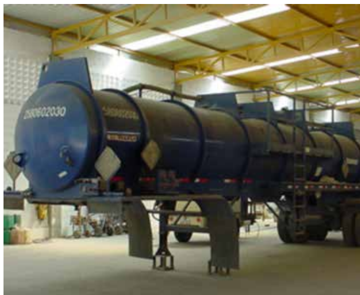
2012 initial application work with two coats of ChemLine® 784/32. First, a grey base coat followed by a red top coat.
