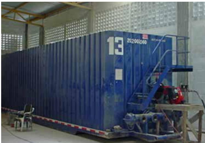
(Top) Fracking tank being readied for internal lining application of ChemLine® 784/32. (Bottom) Inspecting the ChemLine® 784/32 protective coating.
