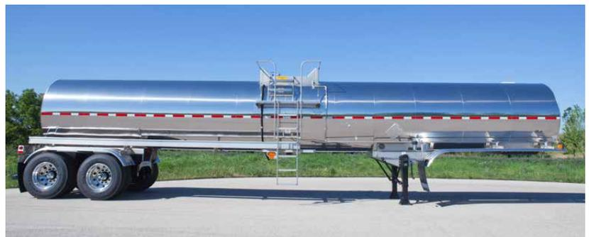
*Typical chemical over-the-road tanker lined with ChemLine® 784/32 provides excellent chemical resistance carrying Sulfuric Acid in concentrations between 50-98%, and other chemicals.*
